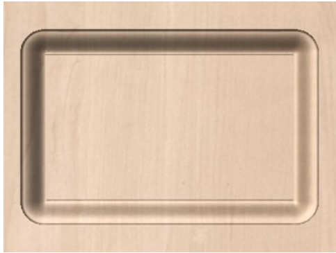
Moulding Toolpath - Create Sharp Corners Un-Checked
