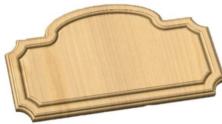
Profile Cutting Strategy with Form cutter
