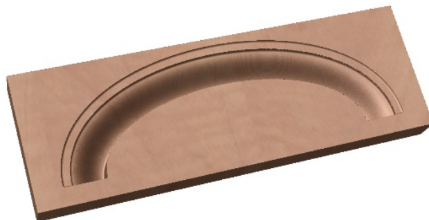
Preview of toolpath created from the cross section and drive rail shown on the previous page.
