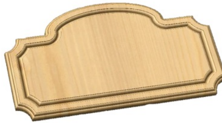
Profile Cutting Strategy with Form cutter
