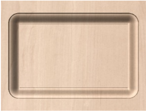
Moulding Toolpath - Create Sharp Corners Un-Checked
