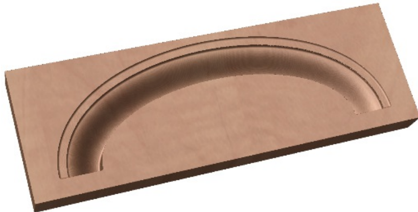
Preview of toolpath created from the cross section and drive rail shown on the previous page.
