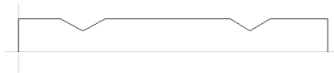
Vector Cross Section to Spin around Left End Point
