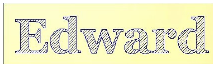
Fill engraving with 45° Hatch pattern
