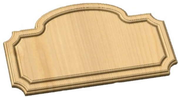
Profile Cutting Strategy with Form cutter
