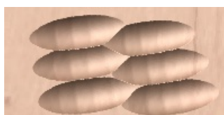
Ramp at start and end switched on
