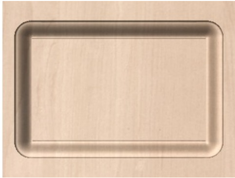
Moulding Toolpath - Create Sharp Corners Un-Checked
