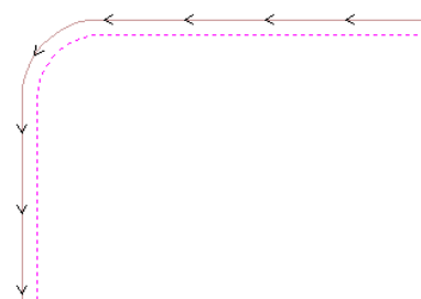
Profiling the Left of the vector using Conventional cutting
