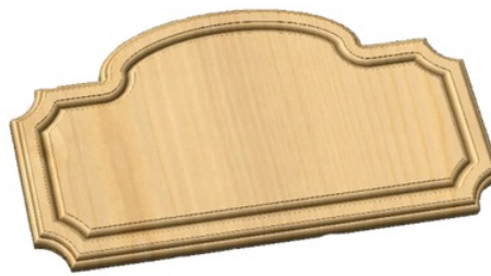
Profile Cutting Strategy with Form cutter
