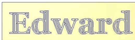
Fill engraving with Offset pattern
