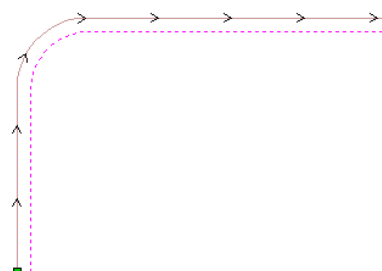
Profiling the Left of the vector using Climb cutting.
