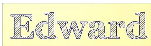
Fill engraving with 45° Hatch pattern
