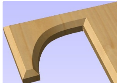
Sharp internal corners selected
