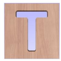
When creating an Inlay toolpath the radius is automatically compensated for, so it is very important to make sure you specify the same tool for both parts of any inlay (male and female). If you do not do this the Inlay will not fit together.
