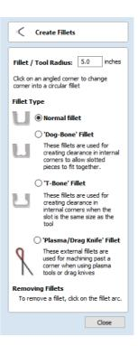
**Note:** Fillets can only be added to spans that are part of the same vector and as such connected, you cannot fillet between two separate vector shapes.
