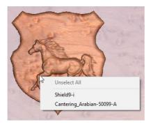
When you RIGHT click on a component without selecting it first the menu will display the names of the components that are positioned at the point your cursor is within the job space. Selecting the name of the component will select it and open up the Properties form for that selected component.
