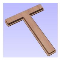
The image shown above shows a Stepped Male Inlay created in 1 inch thick material with a 0.75 inch Step Depth and a 0.3 inch Step Width.
